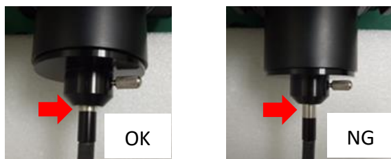
Figure 6: Connect the light guide pipe to the collimating mirror
